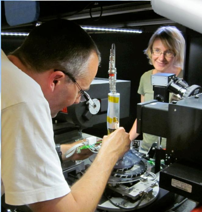
The mass uptake of  $\text{NH}_3$ , the temperature and the 3D structure of AdAmmine were measured during saturation at the DTU Imaging Facility.
