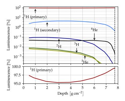
**Figure 5.6:** ExcitonQuenching calculations of the contribution to the total luminescence from each of the six ions based on eq. (5.3). The lower figure is a close-up of the luminescence from the primaries and shows that more than 95% of the total luminescence arises from the protons at any water depth. Figure modified from paper IV.
