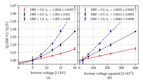
**Figure V.3:** The collected charge  $Q_c$  for the 5 voltages normalized to the charge collected at 200 V for 226 MeV protons at DCPT. The recombination correction factors  $k_s$  (with 1 standard deviation statistical uncertainties estimates from the fits) given in the legends are obtained from extrapolation using (a) a quadratic fit and (b) a linear fit.
