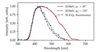
**Figure 2.7:** An optical fibre irradiated at two angles  $\varphi_1$  and  $\varphi_2$  with 20 MeV electrons and with an kV x-ray source below the Čerenkov energy threshold. Figure from paper I.
