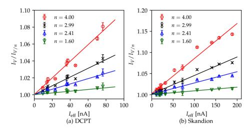
**Figure V.5:** Relative charge collection as a function of the effective current measured at (a) DCPT and (b) the Skandion Clinic. The Boutillon theory in eq. (V.4) has been fitted to all data in each case.
