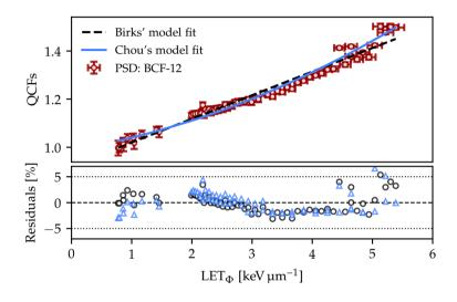
**Figure 4.2:** Quenching correction factors calculated as the ratio of the ionization chamber response to the PSD response in figure 4.1 plotted as a function of the LET<sub> $\Phi$ </sub>. The analyses are truncated at the 80 % distal dose point. The Birks model in eq. (4.2a) and Chou model in eq. (4.2b) are fitted to the data. The lower figure shows the residuals of the experimental data to the Chou model (triangles) and the Birks model (circles).
