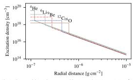
**Fig. 1.** Close-up of the track structures of five ions with  $dE/dx = 30 \text{ keV}\mu\text{m}^{-1}$  in the Pilot-U scintillator modelled as suggested by Chatterjee and Schaefer (1976).
