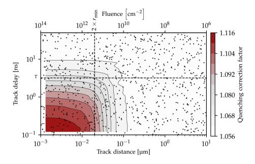
**Figure 5.8:** The total QCF for two 100 MeV proton tracks in the BCF-12 scintillator calculated with ExcitonQuenching. The map is obtained through interpolation of multiple calculations illustrated with dots. The distance between the track centres is varied along with the time between the hits. The quenching is enhanced as the two hits approach each other in time and space. Figure modified from paper IV.
