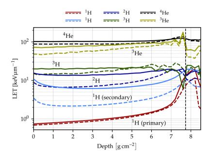
**Figure 5.5:** Geant4 calculations of the LET<sub> $\Phi$ </sub> (dashed lines) and LET<sub>D</sub> (solid lines) for primary and secondary protons as well as the two most common isotopes of hydrogen and helium. The dashed vertical line shows the 80% distal dose point. Figure from paper IV.
