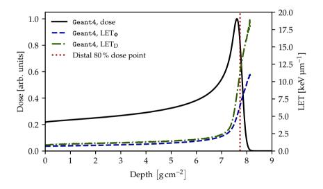
**Figure 3.1:** The Geant4 simulations of the dose deposition (left ordinate) and  $LET_{\Phi}$  and  $LET_{D}$  (right ordinate) in water irradiated with a 100 MeV proton beam.
