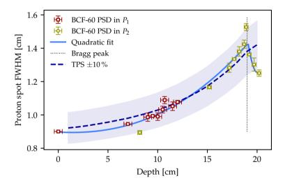
**Figure 6.10:** The FWHM calculated with the two BCF-60 PSDs placed in positions  $P_1$  and  $P_2$  in figure 6.1. Two quadratic fits have been fitted to the data at either side of the approximate location of the Bragg peak. The TPS at DCPT was used to estimate the FWHM shown with a dashed line and 10% uncertainty.
