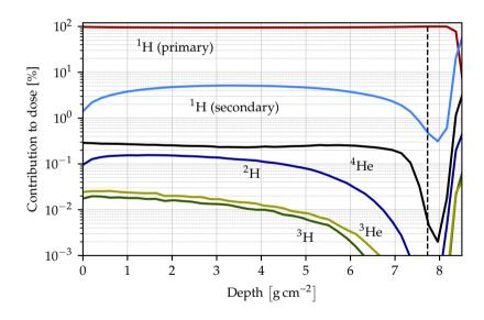
**Figure 5.4:** Geant4 simulations of the dose contribution from six ions in a water phantom irradiated with 100 MeV protons. The dashed vertical line denotes the 80 % distal dose point. Figure modified from paper IV.
