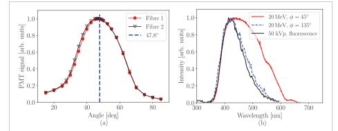
**Figure 2.** (a) PMT signal as a function of gantry angle as optical fibres are irradiated with 20 MeV electrons along with the theoretical emission angle in the fibre core (dashed line). (b) The fluorescence spectrum of the optical fibre obtained with a 50 kVp x-ray source, along with spectra from irradiations using 20 MeV electrons at  $\phi = 45^{\circ}$  (Čerenkov dominated spectrum) and  $\phi = 135^{\circ}$  (fluorescence spectrum) with angles chosen as in figure 1(b).
