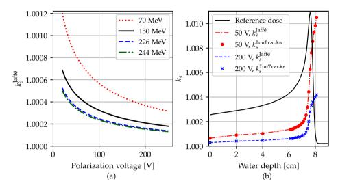
**Figure V.1:** (a) The correction for initial recombination as predicted by the Jaffé theory in a parallel-plate chamber with 2 mm electrode spacing for the relevant proton energies and chamber voltages. (b) The correction factor for initial recombination in the same air-filled IC along the central axis of a 100 MeV proton beam in water calculated with the Jaffé theory (lines) and IonTracks (markers) for 2 polarization voltages. The dose is shown in (b) for reference.
