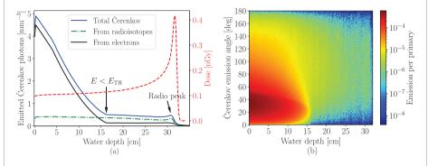
**Figure 5.** GEANT4 simulations of 225 MeV protons in water. (a) The majority of the Čerenkov radiation arises from liberated electrons with a spatial distribution different from the dose, although a minor radiopeak is observable at the Bragg peak. (b) Angular distribution of the emitted Čerenkov photons scored in a 500  $\times$  500 grid relative to the beam direction reveals a broader emission distribution than in electron beams.
