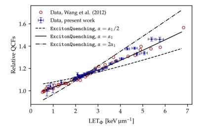
**Figure 4.4:** Experimentally obtained quenching correction factors for the BCF-12 PSD for protons at different energies: data from Wang, Perles, et al. (2012) (circles) and own measurements (markers with errorbars). The theoretical correction factors (lines) are calculated with ExcitonQuenching for different values of the bimolecular quenching parameter  $\alpha$  where  $\alpha_1 = 9.0 \times 10^{-8} \text{ cm}^3 \text{ s}^{-1}$  to illustrate its importance.
