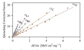
Fig. 2. The quenching correction factor as a function of LET for five ions is calculated with ExcitonQuenching plotted with symbols. The Birks model is fitted to each set of data shown with solid lines.
