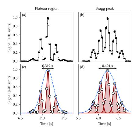
**Figure 6.9:** Subfigures (a) and (b) show the PMT integrated luminescence response from the scintillator measured at the entry channel and Bragg peak region, respectively. An algorithm is used to locate the different plateaus as beam spots plotted with circles in (c) and (d). Gaussians fitted (dashed blue lines) to each of the maxima of the spot lines (red Gaussians) allow an estimate of the FWHM as a time.
