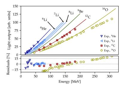
**Figure 5.2:** The ExcitonQuenching predicted luminescence response (solid lines) versus the experimentally measured (markers) luminescence in the Pilot-U scintillator irradiated with several ions stopped in the scintillating material. The experimental data is extracted from Buenerd et al. (1976). The figure is modified from paper III.
