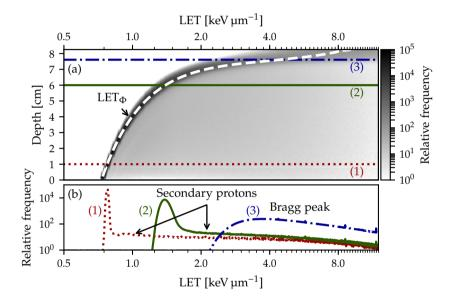
**Figure 5.7:** Geant4 simulated LET spectrum for primary and secondary protons. The upper figure shows the LET as a function of water depth plotted on the left ordinate. The arithmetic mean of the LET spectrum at each depth, the LET<sub> $\Phi$ </sub>, is plotted with a white, dashed line. The lower figure shows the LET spectrum at three depths indicated above with the same line styles. Figure modified from paper IV.
