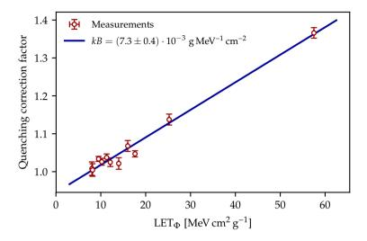
**Figure 6.8:** The measured QCFs from figure 6.7 as a function of the Geant4 calculated LET<sub> $\Phi$ </sub> from figure 6.6. A linear fit normalized to the measurement with the lowest LET<sub> $\Phi$ </sub> is fitted to the data where the slope corresponding to the Birks quenching parameter *kB* is given in the legend.
