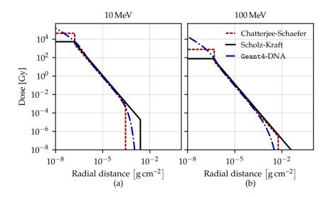
**Figure 3.2:** Radial dose distributions using the analytical Chatterjee-Schaefer ATSM (dashed line) in eq. (3.9), the Scholz-Kraft ATSM (solid line), and Geant4-DNA calculations (dashed-dotted line) for a (a) 10 MeV and (b) 100 MeV proton in water. The Geant4-DNA calculations are extracted from Wang and Vassiliev (2017).
