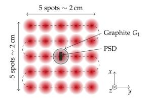
**Figure 6.3:** The spot scanning pattern with a 5 mm spot separation approximately drawn to scale. The PSD and graphite core  $G_1$  at position  $P_2$  where the PSD axis is aligned perpendicular to the beam axis. The diameter of the large graphite disc  $G_2$  exceeds the field size.
