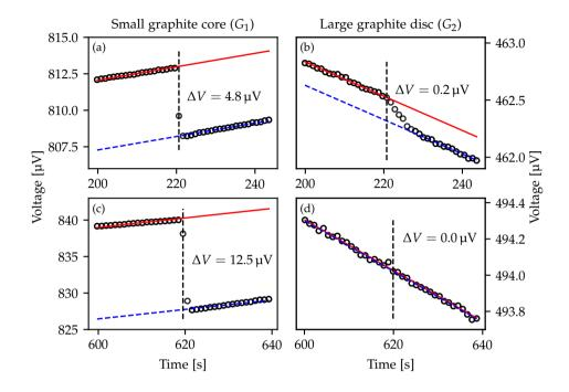
**Figure 6.5:** The response of the smaller graphite core in (a) and the larger in (b) correspond to measurements at the plateau region. (c) is a measurement with the small graphite core  $G_1$  near the Bragg peak and (d) is further downstream behind the distal edge with the graphite disc  $G_2$ . The vertical dashed lines indicate the start of the irradiation.
