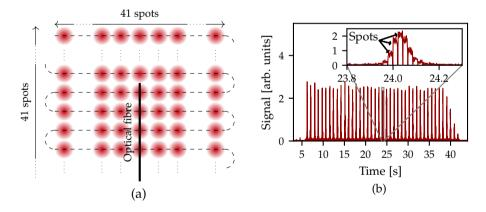
**Figure 2.4:** The pencil beam scans (dashed line) over the optical fibre (solid line) in (a) which gives rise to a signal detected at the PMT. The PMT signal is shown in (b) where each peak corresponds to a horizontal scan line in (a). Figures from paper I.
