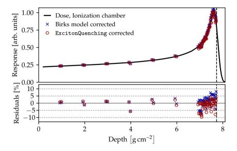
**Figure 5.3:** A quenched PSD response in a 100 MeV proton beam measured at the Skandion Clinic. The quenched signal has been corrected with fits from the Birks model (crosses) and independent predictions by ExcitonQuenching (open circles). The residuals are for each model calculated relative to an ionization chamber measurement. Figure adapted from paper IV.
