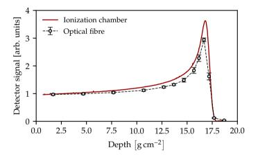
**Figure 2.5:** The luminescence response of the bare optical fibre (k = 2 statistical uncertainties) and an ionization chamber measurement in a water phantom irradiated with 180 MeV protons. Figure adapted from paper I.
