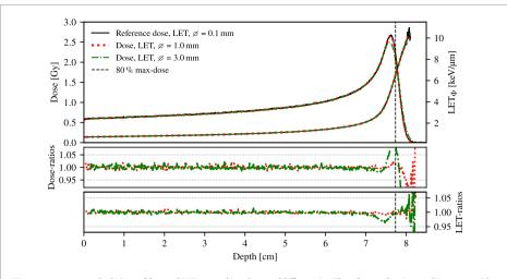
Figure A1. Geant 4 calculations of dose and LET $_{\Phi}$  scored in volumes of different size. The reference dose is scored in 0.1 mm wide voxels. The ratios between the dose and LET $_{\Phi}$  scored in 1 mm and 3 mm diameter voxels to the reference calculations are shown in the two lower figures.
