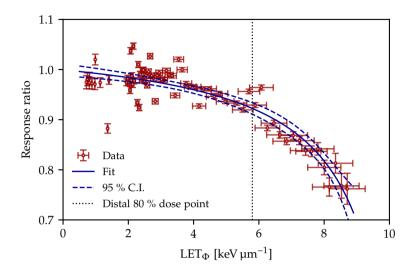
**Figure 5.9:** The ratio of the quenched response of BCF-12 PSD to the quenched response of the 81-0084 fibre as a function of the LET<sub> $\Phi$ </sub>. The 95% confidence interval (C.I.) is shown with dashed lines. The 80% dose threshold is delineated with a dotted vertical line.
