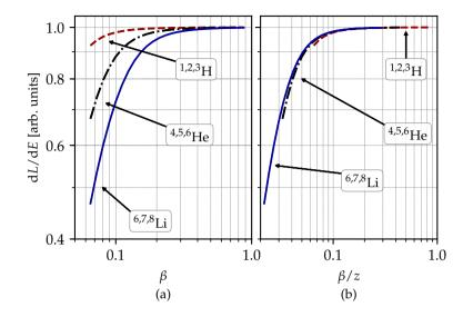
**Figure 5.1:** Luminescence efficiency for isotopes of hydrogen (dashed lines), helium (dashed-dotted lines), and lithium (solid lines) as a function of (a) the relative speed  $\beta$  and (b)  $\beta$  divided by the projectile charge *z*. Figure adapted from paper III.
