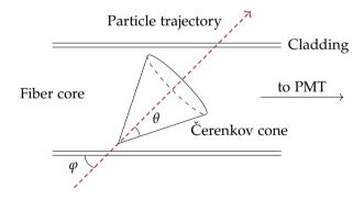
**Figure 2.6:** A charged particle traversing the optical fibre at an angle  $\varphi$  relative to the fibre axis emits Čerenkov radiation at an angle  $\theta$  with respect to the trajectory (dashed line). The fraction of Čerenkov photons guided to the PMT is highly angle dependent.
