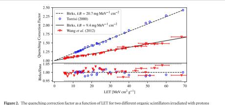
Figure 2. The quenching correction factor as a function of LE1 for two different organic scintillators irradiated with protons where the Birks model is fitted to the data in both cases. The ratios of the QCF obtained from the Birks model to the experimentally obtained values in the figure below indicate a good agreement for both measurements.
