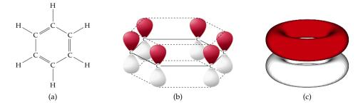
**Figure 2.1:** (a) Diagram of the planar benzene molecule. (b) The  $\pi$ -electrons responsible for the luminescence of the molecule constitute the parallel rings illustrated in (c) where they are free to move. Adapted from (Birks 1964).
