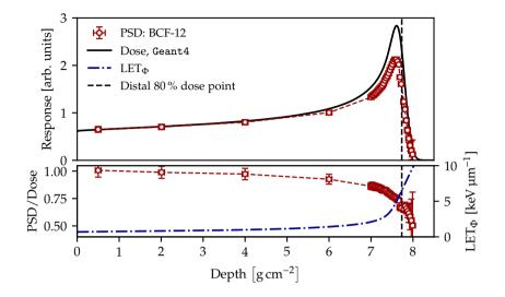
**Figure 4.1:** The Geant4 simulated ionization curve and measured PSD response in a 100 MeV proton beam in water. The ratio of the PSD response to the energy deposition is shown in the figure below on the left ordinate (connected with a dashed line), where the  $LET_{\Phi}$  is plotted for reference with a dot-dashed line on the right ordinate.
