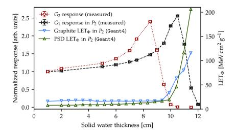
**Figure 6.6:** The measured response of the small and large graphite cores as a function of the solid water width *L*. The LET is scored in Geant4 in both the PSD and the graphite core  $G_1$  in  $P_2$  in two separate simulations.
