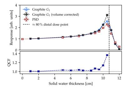
**Figure 6.7:** The response of the PSD and graphite in  $P_2$  versus the SW thickness. The graphite response has been corrected for the volume averaging with eq. (6.4). The QCF (lower figure) has been calculated as the ratio of the volume corrected graphite response to the PSD response.
