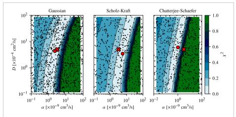
**Figure 4.** Maps over  $\chi^2$  from equation (4) for various values of  $(\alpha, D)$  for the three track structure models. Each dot represents a pair of  $(\alpha, D)$  drawn from a uniform distribution. Only a fraction of the samples are shown. The literature value is marked with a cross in each case, whereas the  $(\alpha, D)$  sets providing the best match to the experimental QCFs are marked with a closed circle and listed in table 2.
