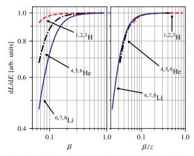
Fig. 4. The scintillation efficiency dL/dE for 3 isotopes of hydrogen, helium, and lithium as a function of (*left*) velocity and (*right*) velocity per atomic number z. All efficiencies coincide in the latter case.
