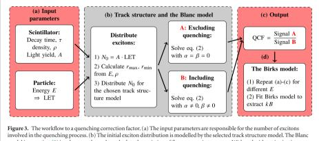
involved in the quenching process. (b) The initial exciton distribution is modelled by the selected track structure model. The Blanc model in equation (2) is subsequently used to calculate the emission of fluorescence in two cases: With and without ionization quenching. (c) The QCF is as a result computed as the ratio of the unquenched to the quenched signal. (d) The Birks model parameter *kB* can be calculated from a fit to a series of the QCFs as a function of LET.
