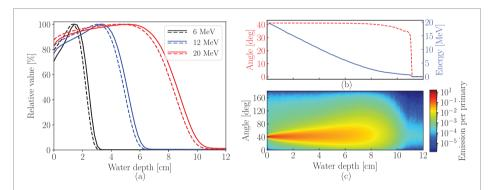
**Figure 3.** GEANT4 simulations of electrons in water. (a) Distribution of dose (solid lines) and emission of Čerenkov photons (dashed lines) for three energies in water. (b) Kinetic energy (solid line) scored along the central axis of a 20 MeV electron beam. The Čerenkov emission angle (dashed line) is plotted as a function of the energy for comparison. (c) Emission angle scored relative to the beam direction.
