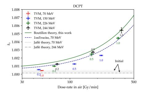
**Figure V.6:** The recombination correction factors  $k_s$  calculated with the TVM (markers) as a function of dose-rate in the IC for the DCPT measurements labelled with the DRF. The Boutillon theory (solid line) is plotted with the DCPT parameters listed in table V.1.
