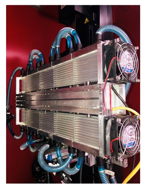
**Figure 3.3:** Picture of five daisy-chained MultiX-ME100 modules with the liquid cooling system and a slit with adjustable aperture size to suppress environmental and scattering noise.
