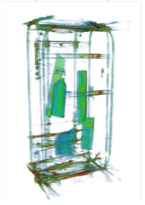
**Figure 5.20:** Input and MAR corrected 3D volume reconstruction of the suitcase at 98.0 keV. The CNN correction removes some of the non-severe streaking artifact introducing however, blurring of the features.
