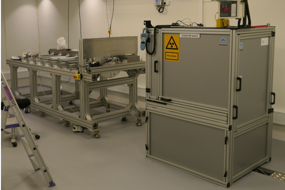
Figure 4.7: Test-rig deployed in front of the ^{60}\text{Co} source.
