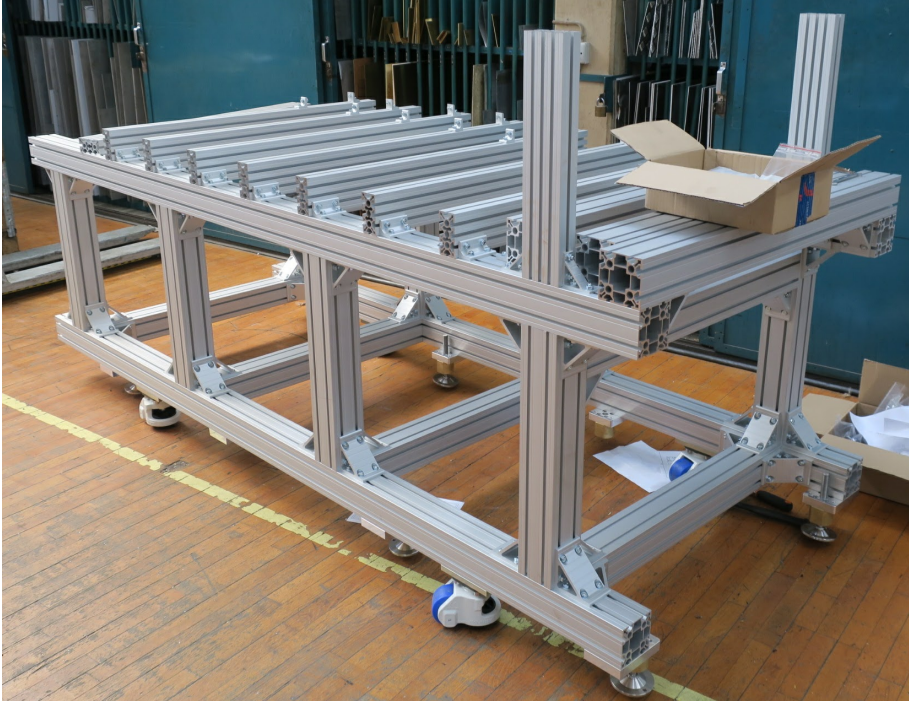
Figure 4.6: Aluminium test-rig structure.
