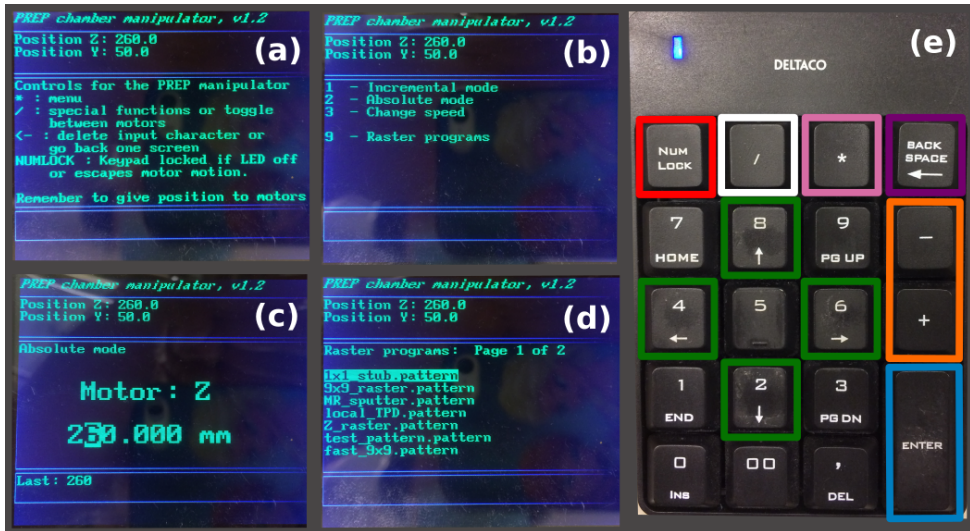
Figure 3.2: User interface for controlling ZY-axis motion of the preparation chamber manipulator using the two stepper motors implemented for rastering. Four main graphical user interfaces feed information back to the user: (a) start-up/splash screen, (b) main menu, (c) motor control - absolute mode, and (d) raster program menu. A keypad (e) feeds user input back to the controller. NumLock (red) is the panic button to abort any unwanted motion as an alternative to pulling the power plug. When the NumLock LED is off, the keypad is also locked to prevent accidental inputs. Remaining highlighted keys are explained in the main text.
