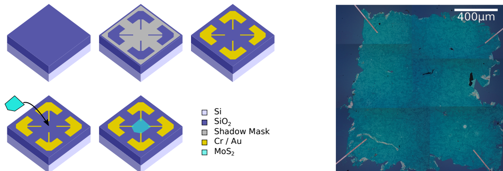
Figure 7.1: (Left) Sketch of the process used to prepare the MoS 2 samples. (Right) microscope picture of a piece of MoS 2 .
