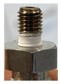
Figure 3.4: Picture of the discoloured Swagelok Part
