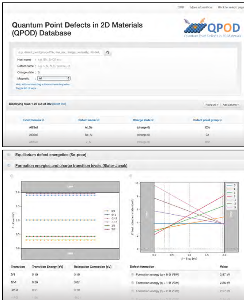
Figure 6.3: The QPOD database web application. Snapshot of the QPOD search interface (top) and an example of the web-panel for charge transition levels and formation energies for the Al Se defect in Al 2 Se 2 (bottom). In the search panel a user can query for predefined parameters (host name, defect name, charge state) or any other KVP inside the QPOD database. The 'Formation energies and charge transition level (Slater-Janak)' web-panel shows both the charge transition levels (bottom, left) as well as the formation energies (bottom, right) in a table and in a figure.
