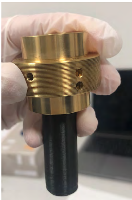
Figure B.1: Center part of the cryogenic cavity, containing the two mirrors and the crystal, shown with the assembling tool (black).
