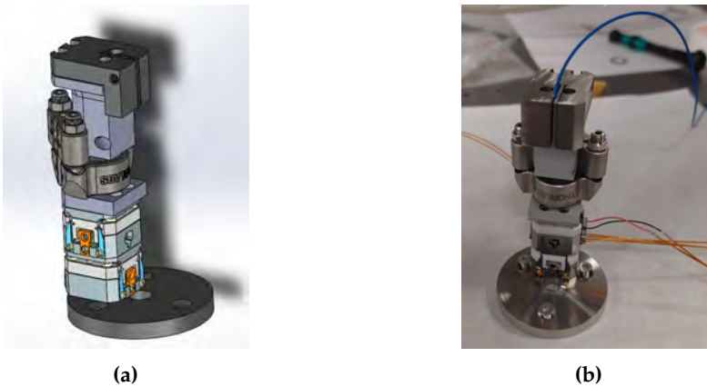
Figure 5.9: In order to get more degrees of freedom (tip-tilt) of the in-coupling light, a modification of the cavity design was performed, constituting a mirror mount and adapters in between x-y-stage and the GRIN lens holder. The modification is shown as a Solidworks model in (a) of the mirror mount (grey) added to the design in between the x-y-stage (light blue) and the GRIN lens holder (dark grey) with adapters (blue) in order to be mounted. The actual components are depicted in (b) with the mirror mount added to the design in between the x-y-stage and the GRIN lens holder.
