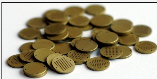
Standard single grain discs with depth and diameter of 300 \mu\text{m} . Picture on the right shows blue stimulated quartz OSL recorded with the EMCCD option (item 304; Thomsen et al., 2015).
