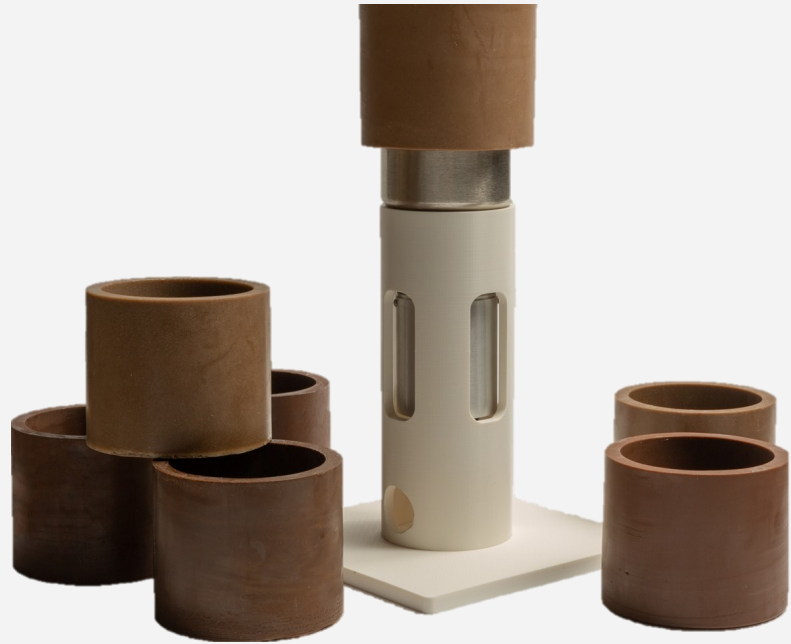
The picture shows the detector placed in the holder with a sample in place for counting.
