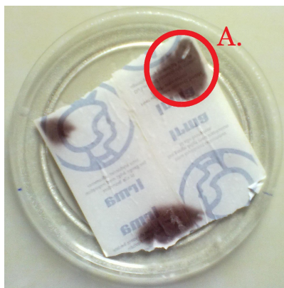
Figure 1: The result of heating wet thermal paper in the micro-oven. Three distinct maxima can be seen as dark spots on the paper. The one labelled A was used for the synthesis process.
