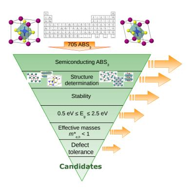
Fig. 1 Sketch of the screening funnel. The different design criteria lead to a gradual reduction in the number of candidate materials.
