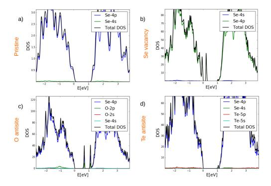
Figure 5: Density of states of pristine selenium structure (a), structure with selenium vacancy (b), oxygen antisite (c) and tellurium antisite(d). Selenium vacancy and oxygen antisite introduce mid-gap states whereas tellurium antisite does not seem to have a significant effect on the band structure.
