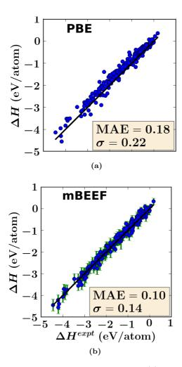
Figure 2.2: Calculated heats of formation with PBE (a) and mBEEF(b) functional. MAE is the mean absolute error and  $\sigma$  is the standard deviation of the difference between calculated and experimental values. Figures from Ref. [50].
