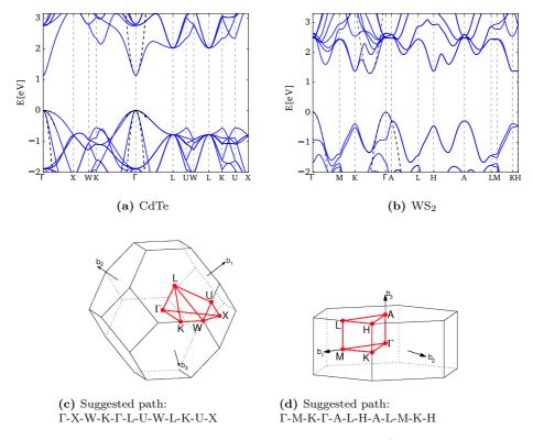
Figure 3.5: Band structures of CdTe in the fcc structure,a), and WS<sub>2</sub> in hexagonal structure, b). Calculations were performed using Setyawan and Curtarolo scheme and the fcc and hexagonal Brillouin zone and the high symmetry path used is shown in c) and d), respectively. Black dashed lines represent parabolic fitting to VBM and CBM. In case of band degeneracy at the extrema, a fitting was produced for each band and equivalent number of effective masses obtained.
