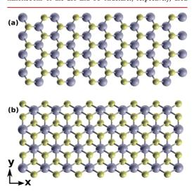
**Figure 6.** (a) Structure of a nanoribbon of the 2H structure cleaved along the nonpolar direction. The edges of the nanoribbons lie along the *x*-axis with a finite width along the *y*-axis; (b) a nanoribbon cleaved from the 1T structure.
