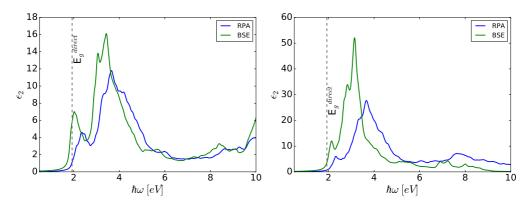
Figure 3: Optical spectra perpendicular (left) and along (right) Se rod direction obtained with BSE (green) and RPA (blue). The vertical lines mark direct band gap position, calculated with GLLB-SC functional.
