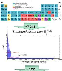
Figure 2: Flow of data selection process: Entries are extracted from the OQMD database (22,807 that originate from the ICSD with up to three elements), only entries containing non-toxic, abundant and low HHI elements are to be considered further. Furthermore, the number of candidates is additionally decreased by selecting only semiconducting materials with 0 eV<  $\mathrm{E}_g^{PBE} \leq 2$  eV, containing up to three elements resulting in 1,630 candidates.
