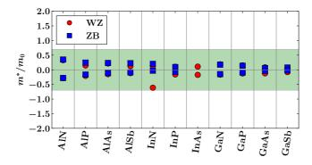
**Figure 6.3:** Calculated effective masses for electrons and holes. The signs correspond to the orientation of the parabola fitted to the top of the valence band (holes) and bottom of the conduction band (electrons).
