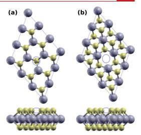
**Figure 1.** (a) Top and sideview of a prototypical structure of a metal dichalcogenide in the 2H structure used for the defect calculations. The unit cell is shown by the dotted lines. The defect structure is created by making a chalcogen vacancy as indicated by a blue ellipse. (b) Similar figure as (a) for the 1T structure.
