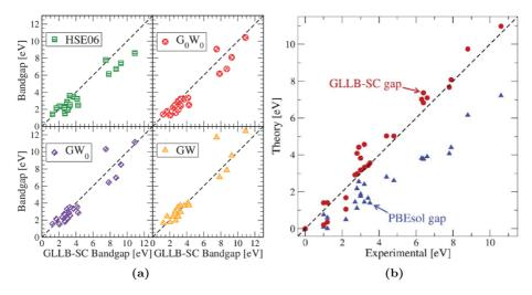
Figure 2.1: a) HSE06, G<sub>0</sub>W<sub>0</sub>, GW<sub>0</sub>, GW band gaps (upper left to bottom right, respectively) as a function of the GLLB-SC gaps. T All the methods except GW underestimate the gaps with respect to the GLLB-SC. b) Comparison between the theoretical and experimental band gap of non-magnetic metal oxides in their most stable structure. Figures from Ref. [36]a) and [37]b).
