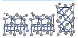
Figure 2. Polytypes of ZnSnN<sub>2</sub>. (a) Wurtzite–kesterite (KT). (b) Wurtzite–stannite (ST). (c) Zincblende–chalcopyrite (CP). Blue, green, and gray spheres represent the nitrogen, tin, and zinc atoms, respectively.
