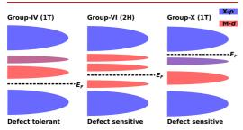
Figure 5. Sketch showing the filling of the electronic levels of the different groups of the transition metal dichalcogenides. The TMDs of group-IV are defect-tolerant, whereas the TMDs of group-VI X are defect-sensitive. The chalcogen p states are shown in blue and the metal d states in red. The regions with mixed color have mixed p and d character.
