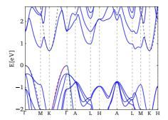
**Figure 3.6:** Band structure of Mg<sub>3</sub>Sb<sub>2</sub>: the valence band shows different curvature in the two different directions, K- $\Gamma$  and  $\Gamma$ -A which yield different effective masses.
