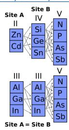
**Figure 1.** Selection of elements for sites A, B, and X. In cases where the elements at site A and site B belong to the same group, the order AB is equivalent to order BA since the sites A and B are equivalent in terms of symmetry.
