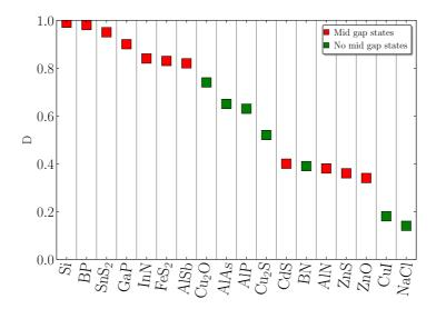
Figure 6.1: NNO descriptor values (D) for investigated bulk compounds. Red squares indicate the compounds manifesting deep defect states and the green squares indicating the compounds showing no deep defect states after the introduction of a vacancy. The energy window of 2eV was used for calculating D.
