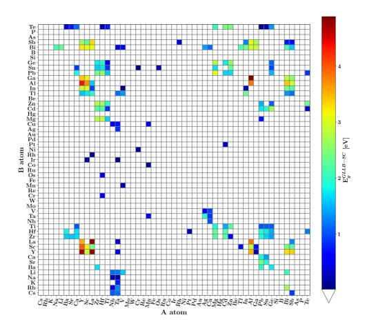
Fig. 2 Calculated band gap values using the GLLB-SC functional for the distorted 5-atom unit cell. Most of the materials do not have a band gap because the valences do not add up to zero. 129 compounds exhibit a band gap in the distorted 5-atom unit cell.
