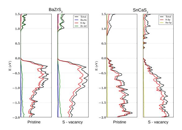
Fig. 6 Projected and total density of states for  $BaZrS_3$  (GdFeO<sub>3</sub> structure)(left) and  $SnCaS_3$  (NH<sub>4</sub>CdCl<sub>3</sub>/Sn<sub>2</sub>S<sub>3</sub> structure)(right) with and without a sulfur vacancy. In the case of  $BaZrS_3$  the introduction of a vacancy does not give rise additional states inside the band gap, while in the case of  $SnCaS_3$ , deep states are found within the band gap.
