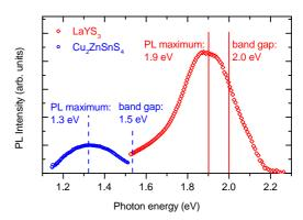
Fig. 9 Photoluminescence spectra of LaYS3 (red) and Cu2ZnSnS4 (blue) thin films. The scale is the same for both spectra. The solid (dashed) vertical lines indicate the PL peak position and band gap of LaYS3 (Cu2ZnSnS4).
