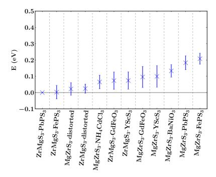
**Figure 2.3:** Comparison of formation energies for ZrMgS<sub>3</sub> compound in several different phases. The uncertainties are calculated with respect to the most stable structure.
