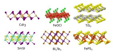
Figure 7.7: Examples of monolayers of some of the most common layered prototypes: CdI<sub>3</sub>, FeOCl, TiS<sub>3</sub> (two layers since the structure has a translational symmetry), SmSI, Bi<sub>2</sub>Te<sub>3</sub> and FePS<sub>3</sub>.
