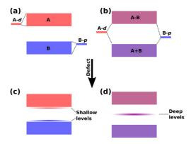
**Figure 4.1:** (a and b) Nature of the band structures near the band edges for the defect-tolerant and defect-sensitive cases, respectively.(c and d) Shallow and deep levels introduced after the creation of defects. Figure from paper I.
