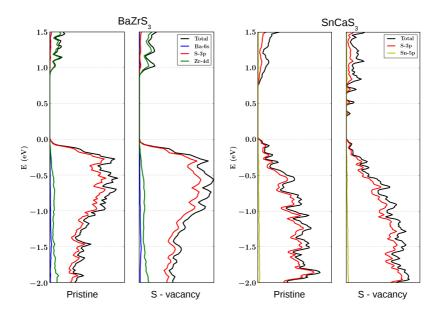
Figure 3.7: Projected and total DOS of BaZrS<sub>3</sub> and SnCaS<sub>3</sub>. Introduction of sulfur vacancy results in additional states in the band gap of SnCaS<sub>3</sub> and the material is called defect sensitive. DOS of BaZrS<sub>3</sub> does not change significantly and no new states are found so the material is defect tolerant. (Here defect tolerance only implies sulfur vacancy so the procedure should be repeated for other types of defects as well.) Figure from Paper III.
