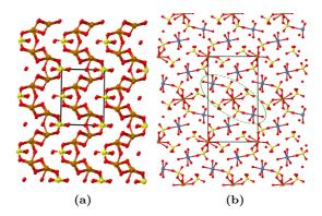
**Figure 7.2:** Low dimensional nature of Na<sub>2</sub>GeO<sub>10</sub> a) and FeO<sub>16</sub>S<sub>2</sub>Zn b). The green ellipse in b) highlights a single 1D rod.
