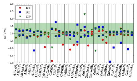
Figure 7. Effective masses for electrons and holes. The negative sign is due to the orientation of the parabola fitted to the top of the valence band; therefore, hole masses have negative sign. Similarly, electron masses have positive sign. Green area is the limit of "light masses". Thick vertical lines are shown to divide the compounds into AB(N, P, As, Sb)<sub>2</sub> group where "AB" is a particular combination of cations.
