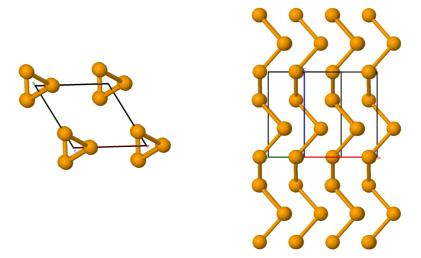
Figure 1: Crystal structure of trigonal Selenium: the one dimensional spiral rods are extending in the c-axis direction (right). The view from the top (left) shows the arrangement of rods in the corners of hexagonal primitive cell.
