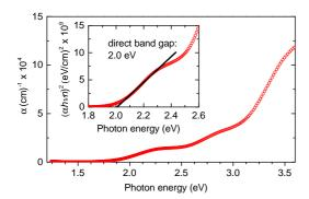
Fig. 8 Main plot: absorption coefficient of LaYS3 according to spectroscopic ellipsometry. Inset: Determination of the value of the direct band gap from absorption coefficient and refractive index 81, both extracted by spectroscopic ellipsometry.
