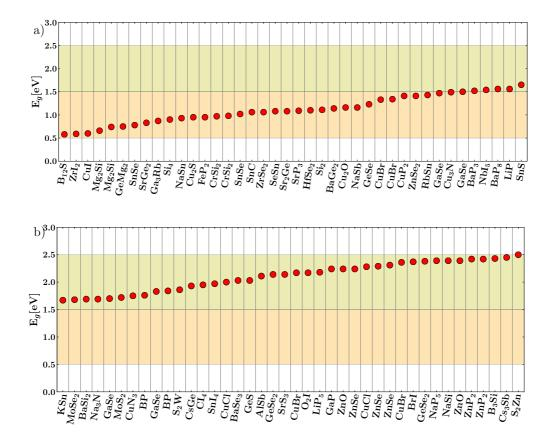
Figure 4: Calculated band gaps of binary systems satisfying the screening criteria for abundance, non-toxicity, light absorption, and mobility. Orange and yellow areas represent LBG and HBG regions, respectively. Table with numerical values and ICSD codes can be found in the supplementary material.
