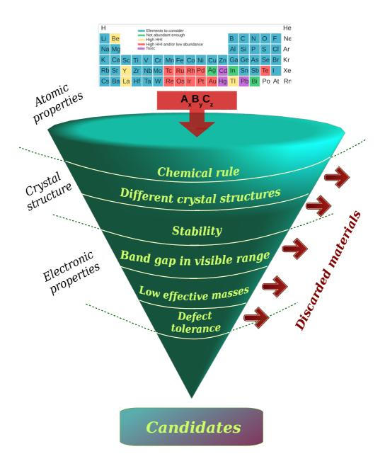
**Figure 3.1:** Illustration of a step-wise screening procedure using funnel annalogy: initial large number of candidates is reduced every time a new property is investigated. As moving towards the bottom of the funner, the number of candidates decreases, and the cost of the DFT calculations increases.
