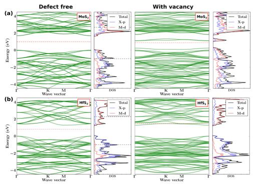
Figure 2. (a)PBE band structures, the DOS, and the PDOS on the chalcogen p-orbitals and metal d-orbitals of the monolayer  $2H-MoS_2$  in its pristine form (left) and with an S vacancy (right). For comparison, the band structure is plotted for  $3 \times 3$  supercell for the pristine as well as the defect structure. The energy levels have been aligned to the valence band maximum of the pristine monolayer. (b) Similar figure as (a) for  $1T-HfS_2$ .
