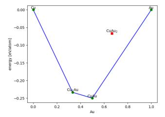
**Figure 3.4:** Example of the convex hull (blue line) calculated for Cu-Au phase space: the green points correspond to the stable materials and the red points to unstable materials. All the points on the convex hull are stable while the ones above the hull are unstable.
