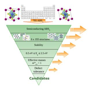
**Figure 4.3:** Illustration of the screening funnel adopting design criteria used in this work. At each stage, a new criteria is introduced and all materials not satisfying it are removed from further consideration. Figure from paper III.
