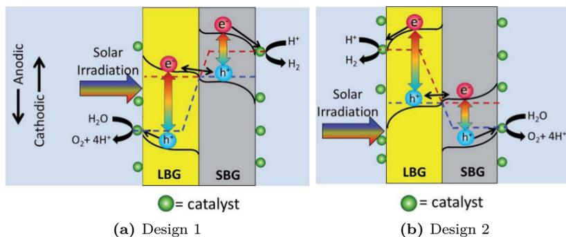
**Figure 1.2:** Proposed designs for a two-photon water splitting device. (a) The large band gap material (LBG) is the photoanode and the small band gap material (SBG) the photocathode. Vice versa in (b), LBG is the photocathode and SBG the photoanode. Figures from reference [13].
