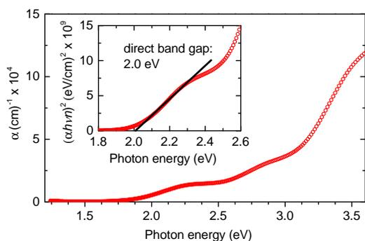
**Fig. 8** Main plot: absorption coefficient of LaYS<sub>3</sub> according to spectroscopic ellipsometry. Inset: Determination of the value of the direct band gap from absorption coefficient and refractive index<sup>81</sup>, both extracted by spectroscopic ellipsometry.
