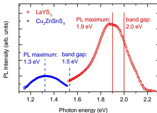
**Fig. 9** Photoluminescence spectra of LaYS<sub>3</sub> (red) and Cu<sub>2</sub>ZnSnS<sub>4</sub> (blue) thin films. The scale is the same for both spectra. The solid (dashed) vertical lines indicate the PL peak position and band gap of LaYS<sub>3</sub> (Cu<sub>2</sub>ZnSnS<sub>4</sub>).
