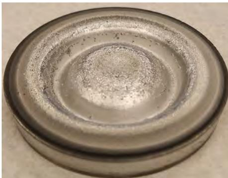
**Figure 2.7:** Picture of a heavily used Ru sputter target (2 inch in diameter and 6 mm thick) showing the "racetrack" pattern of the plasma sputtering.
