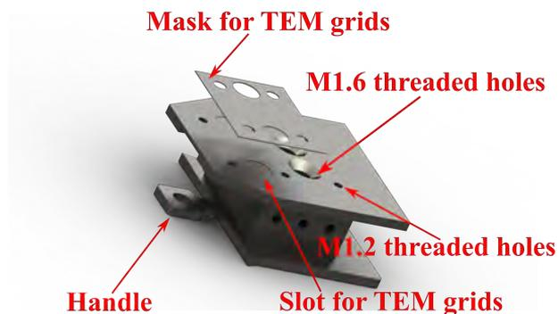
**Figure C.2:** Rendered image of the general use sample holder with the mask for TEM grids. The sample holder is made of stainless steel and has 6 vented threaded holes to attach samples or other extensions with M1.2 screws. The small indents (3.1 mm in diameter and 0.05 mm deep) for TEM grids and the thin stainless steel plate to keep the grids in place are also depicted in the image. The sample holder is kept together with M1.6 screws with sunk heads in vented holes.
