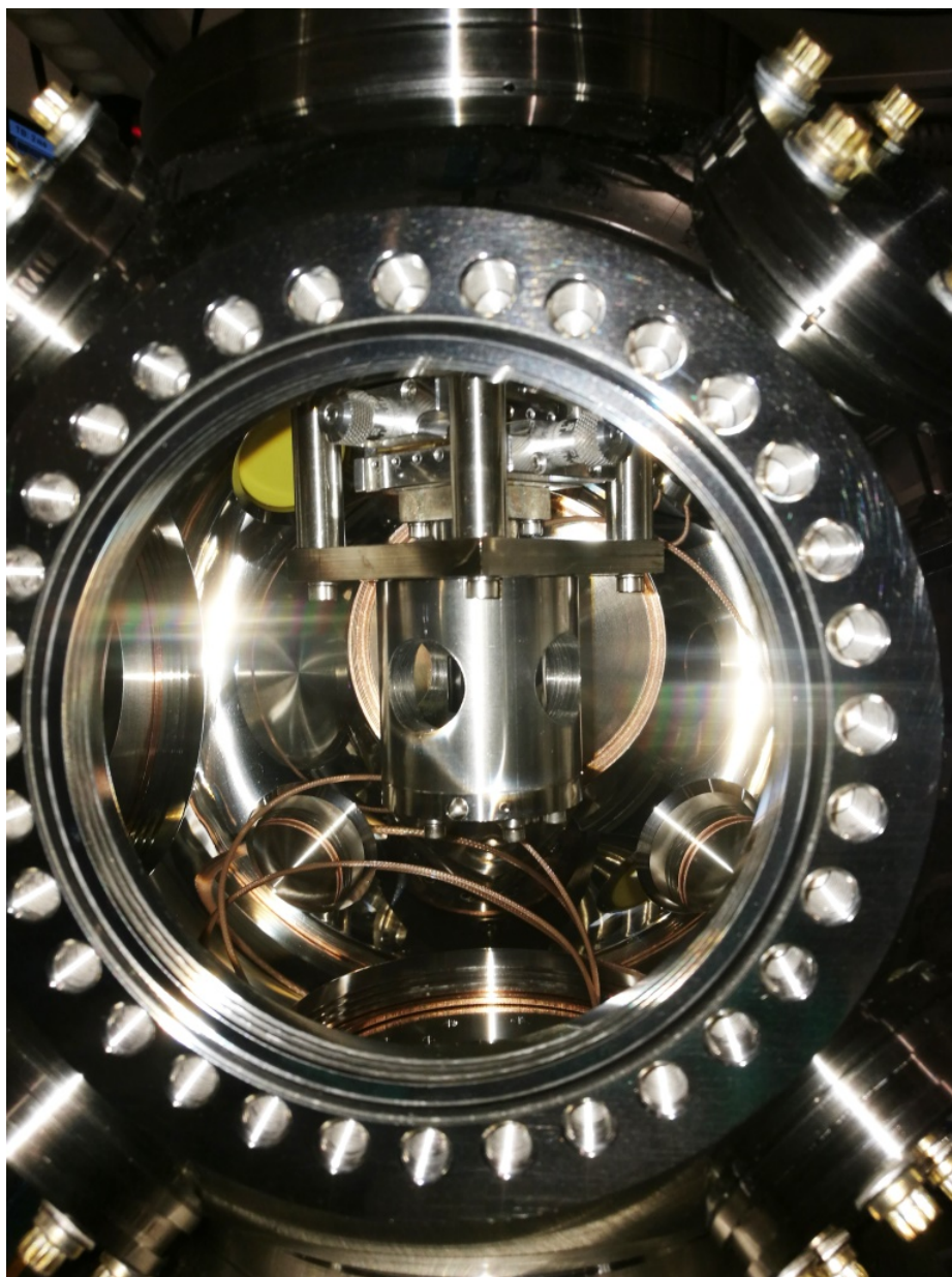
Figure 4.9: View of the optical cavity inside the vacuum chamber.
