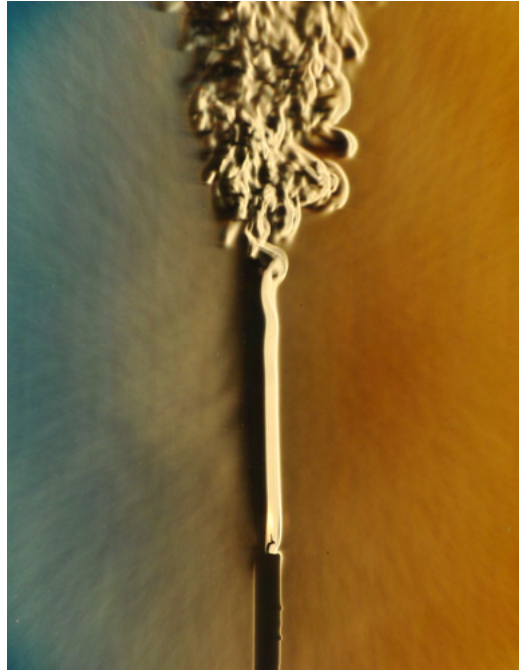
Figure 2.1: The rising plume of a candle in still air. Being initially laminar, the flow develops in a very short transition phase into turbulence in the upper part of the image [8].
