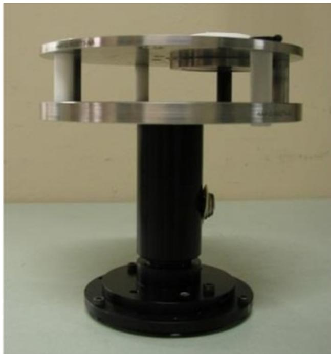
**Figure 6.3:** Picture of the carousel sample holder with six different materials in place. Figure courtesy of Dooraghi et al. [97]
