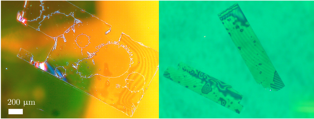
Figure 3.4: Diamond membranes on DBR mirrors imaged using an optical microscope.
