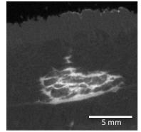
The drug distribution has been visualized with high spatial resolution using the Xradia Versa VRM-410 at DTU.
