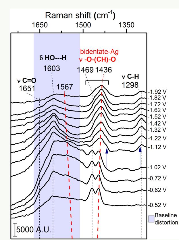
Polycrystalline Ag, during CO<sub>2</sub>ER, in 0.05 M Li<sub>2</sub>B<sub>4</sub>O<sub>7</sub> saturated with CO<sub>2</sub>, bulk pH of 6.1.
