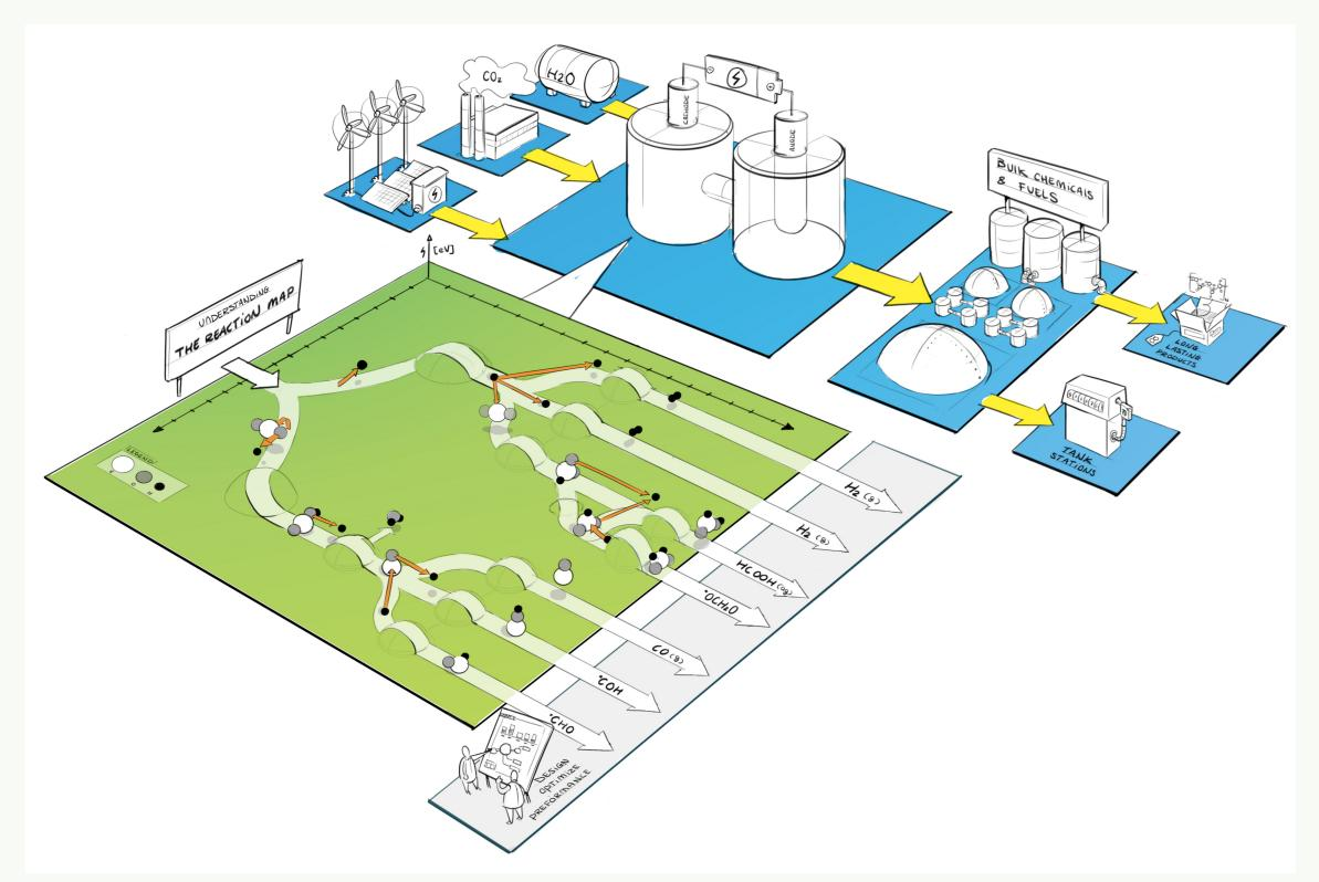
CO and HCOO<sup>-</sup>: 2 CPET products with relatively low overpotentials, high faradaic efficiencies. Ag catalysts: balance of performance with low cost electrodes.
