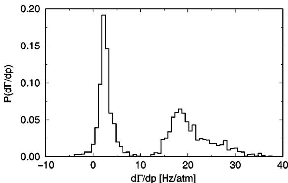
FIG. 9. The distribution of slopes  $d\Gamma/dp$  has two well-separated peaks, which makes it possible to separate the flexural and in-plane modes. We choose a “separation” slope of 11 Hz/atm. A few inaccurate fits give rise to the small number of negative slopes.
