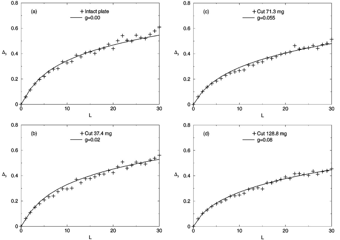
FIG. 14. The  $\Delta_3$  statistic for all the modes is fitted by minimizing the sum of the squared deviations between the data and the random matrix result. (a) The plate is intact. (b) A total of 37.4 mg has been removed. (c) A total of 71.3 mg has been removed. (d) A total of 128.8 mg has been removed.
