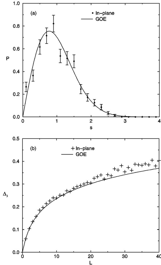
FIG. 11. The level spacing distribution (a) and the  $\Delta_3$  statistic (b) for the in-plane modes compared with the GOE statistics. The  $\Delta_3$  statistic shows that the spectrum of the in-plane modes is slightly less rigid than the GOE.
