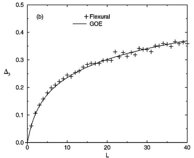
FIG. 10. The level spacing distribution (a) and the  $\Delta_3$  statistic (b) for the flexural modes compared with the GOE statistics. Both the level spacing distribution and the  $\Delta_3$  statistic agree very well with the GOE results.
