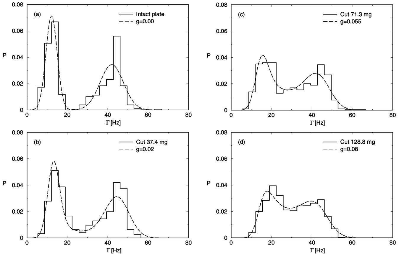
FIG. 15. The experimental width distribution for the resonances compared to the distribution  $P(\Gamma)$  obtained numerically using Eq. (3). The three plots represent data for the same slit depths and values of  $g$  as in Figs. 13 and 14. (a) The plate is intact. (b) A total of 37.4 mg has been removed. (c) A total of 71.3 mg has been removed. (d) A total of 128.8 mg has been removed.
