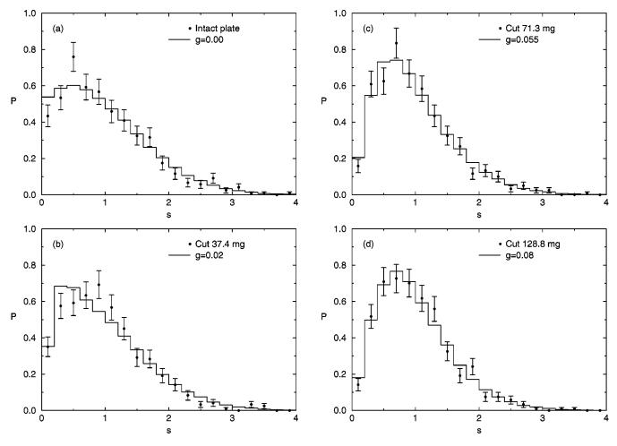
FIG. 13. The level spacing distribution for all the modes compared to the result of the random matrix model. (a) The plate is intact. (b) A total of 37.4 mg has been removed. (c) A total of 71.3 mg has been removed. (d) A total of 128.8 mg has been removed.
