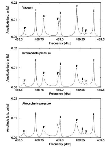
FIG. 6. A segment of the resonance spectrum for the 2-mm-thick three-leaf clover at three different pressures: vacuum, 0.5 atm, and 1 atm. Most resonances are easily recognized to be either in-plane (I) or flexural (F).
