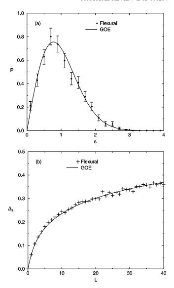
FIG. 10. The level spacing distribution (a) and the  $\Delta_3$  statistic (b) for the flexural modes compared with the GOE statistics. Both the level spacing distribution and the  $\Delta_3$  statistic agree very well with the GOE results.
