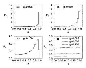
FIG. 4. The asymmetry distribution  $P_A(a)$  obtained numerically for random matrix ensembles with  $N_1 = N_2$ . The value  $P_A(0)$  grows linearly with g, see the blow-up on (d), as predicted in the simple analytical model of the eigenvector mixing, see Eq. (8).
