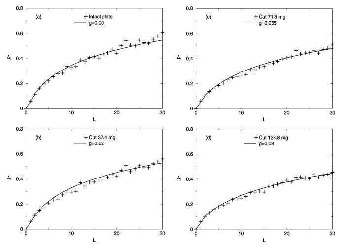
FIG. 14. The  $\Delta_3$  statistic for all the modes is fitted by minimizing the sum of the squared deviations between the data and the random matrix result. (a) The plate is intact. (b) A total of 37.4 mg has been removed. (c) A total of 71.3 mg has been removed. (d) A total of 128.8 mg has been removed.
