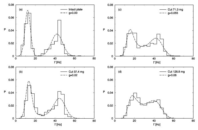
FIG. 15. The experimental width distribution for the resonances compared to the distribution  $P(\Gamma)$  obtained numerically using Eq. (3). The three plots represent data for the same slit depths and values of g as in Figs. 13 and 14. (a) The plate is intact. (b) A total of 37.4 mg has been removed. (c) A total of 71.3 mg has been removed. (d) A total of 128.8 mg has been removed.
