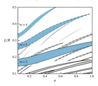
FIGURE 3. (Colour online) Stability map in the parameter space  $(a, \xi/R)$  for m=2(plain lines), m=3 (dotted lines) and m=4 (no lines). Coloured areas correspond to positive growth rate. The main resonances are shown in blue. A small amount of viscous dissipation is introduced with  $C = 10^{-4}$  to filter out high-order secondary resonances (see appendix B).
