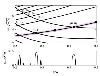
FIGURE 7. (Colour online) Normalized frequencies  $\omega_r \sqrt{R/g}$  and growth rates  $\omega_i \sqrt{R/g}$ from global stability as a function of  $\xi/R$  for a=0.7 and m=3. Along  $G_0$  branch which is highlighted, black squares correspond to mode structures reported in figure 8.
