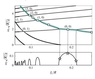
FIGURE 9. (Colour online) Normalized frequencies  $\omega_r \sqrt{R/g}$  and growth rates  $\omega_i \sqrt{R/g}$ from global stability as a function of  $\xi/R$  for a=0.3 and m=2. Along  $C_0$  branch which is highlighted, empty squares (respectively stars), correspond to mode structures reported in figure 10 (respectively figure 11).
