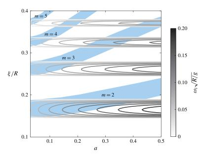
FIGURE 13. (Colour online) Instability map for the main resonance (0, 0) and for m=2, 3, 4 and 5. Comparison between the numerical solution of the shallow-water equation, (4.4), (contours of normalized growth rate are shown in grey scales) and the instability map obtained from the global stability approach detailed in § 2 (blue zones).
