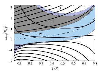
FIGURE 16. (Colour online) Normalized frequencies  $\omega_r \sqrt{R/g}$  as function of  $\xi/R$  for m=5 and a=0.01. Superposition of global stability results (black thick lines) and areas corresponding to the different configurations presented in figure 15. Legends and colours conventions are identical to figure 15.
