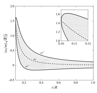
FIGURE 14. Epicyclic frequencies obtained for a = 0.01 and  $\xi/R = 0.1$ . Thick lines correspond to the normalized epicyclic frequencies  $(\omega^{\pm}/m)\sqrt{R/g}$  given by (4.7), dashed line corresponds to the normalized critical frequency  $(\omega_c/m)\sqrt{R/g}$ . Grey area corresponds to  $\Lambda > 0$  (evanescent behaviour), white areas to  $\Lambda < 0$  (oscillatory behaviour). The inset shows a magnification near  $r = \xi$ .
