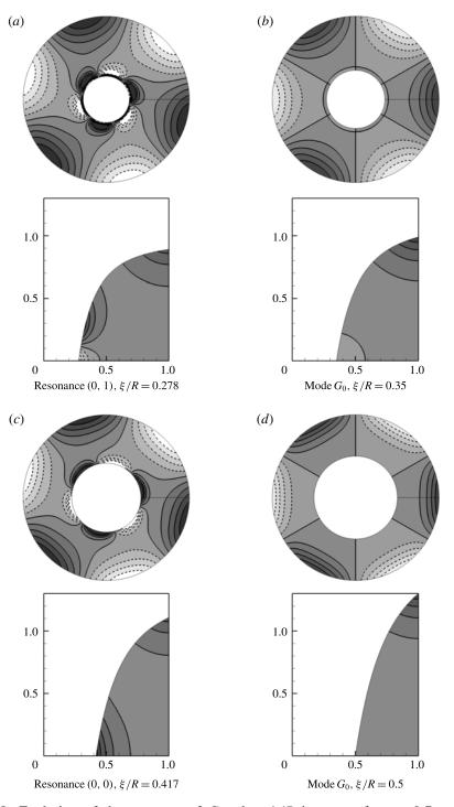
FIGURE 8. Evolution of the structure of  $G_0$  when  $\xi/R$  increases for a=0.7 and m=3. The corresponding frequency evolution is highlighted in figure 7 and the structures shown here correspond to the black squares on figure 7. Contours and colour conventions are the same as in figure 5.
