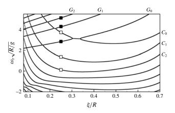
FIGURE 4. Normalized frequencies  $\omega_r \sqrt{R/g}$  as a function of  $\xi/R$  for a = 0.3 and m = 3. Squares at  $\xi/R = 0.25$  correspond to mode structures shown in figure 5 (filled symbols) and figure 6 (empty symbols).
