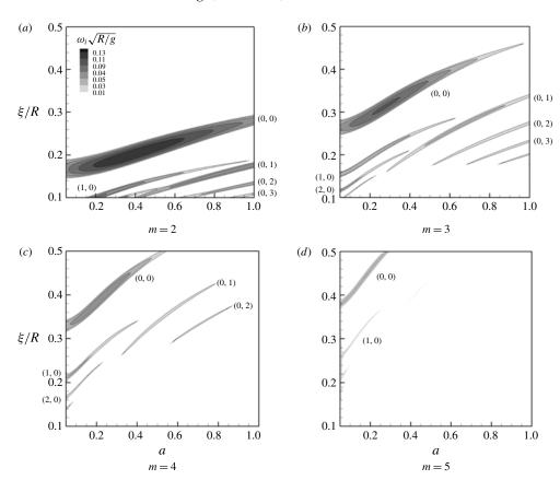
FIGURE 2. Stability maps in the parameter space  $(a, \xi/R)$  for different values of m. Grey levels correspond to normalized growth rate contours  $(\omega_i \sqrt{g/R})$ . A small amount of viscous dissipation is introduced with  $C = 10^{-4}$  to filter out high-order secondary resonances (see appendix B).
