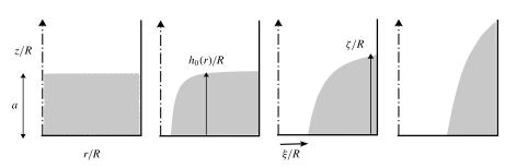
FIGURE 1. Typical free-surface shapes (2.4c) obtained for a given fluid volume and increasing values of  $\xi/R$  from left to right:  $\xi/R \to 0$ ,  $\xi/R = 0.1$ ,  $\xi/R = 0.3$ ,  $\xi/R = 0.5$ .
