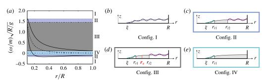
FIGURE 15. (Colour online) (a) Epicyclic frequencies obtained for a = 0.01 and  $\xi/R = 0.1$  (same as figure 14) where the different possible configurations depending upon the frequency values are shown in colours. The horizontal lines from top to bottom respectively correspond to  $\max(\omega^+(r))$  (dotted),  $\omega_c(\xi)$  (dashed),  $\omega^+(R)$  (plain),  $\omega_c(R)$  (dashed),  $\omega^-(R)$  (plain) and min( $\omega^-(r)$ ) (dotted). (b-e) Sketches of the obtained configurations.
