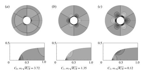
FIGURE 6. Example of centrifugal modes for a = 0.3, m = 3 and  $\xi/R = 0.25$  (empty squares in figure 4). Contours and conventions are the same as in figure 5. All the displayed structures correspond to neutral waves  $(\omega_i \sqrt{R/g} = 0)$ .
