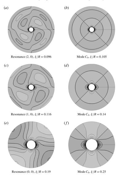
FIGURE 10. Evolution of the structure of  $C_0$  when  $\xi/R$  increases for a = 0.3 and m = 2. The corresponding frequency evolution is highlighted in figure 9 and the structures shown here correspond to the black empty squares on figure 9. Only velocity potential contours from the top view representation are shown here. Conventions are identical to figure 5.
