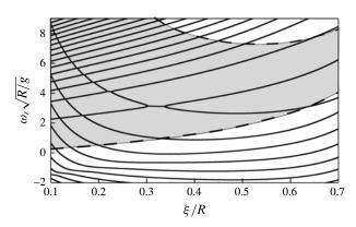
FIGURE 12. Normalized frequencies  $\omega_r \sqrt{R/g}$  as a function of  $\xi/R$  for a=0.3 and m=3. The shaded area between dashed lines shows the region where a critical radius is present in the fluid domain, i.e.  $\xi < r_c < R$ . Upper dashed line corresponds to  $\omega_r = m\Omega(\xi)$  (critical radius at  $r = \xi$ ), lower dashed line corresponds to  $\omega_r = m\Omega(R)$  (critical radius at r = R).
