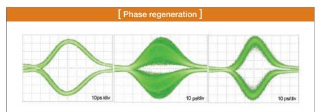
Data without phase noise (left), with added phase noise before regeneration (middle) and with added phase noise after regeneration (right). From K. Croussore et al. Opt. Express **13**, 3945-50 (2005).
