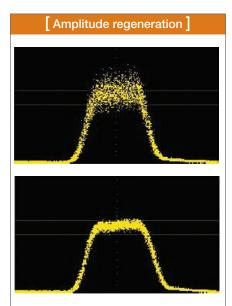
Pumps at 1,567 and 1,604 nm, and a signal at 1,583 nm, produced primary and secondary idlers at 1,587 and 1,576 nm, respectively. Power profile of the noisy input signal (top) and power profile of the regenerated secondary idler (bottom).
