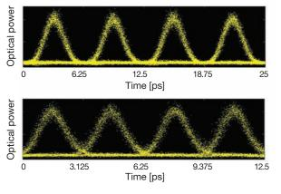
Measured eye diagrams of 160-Gb/s (top) and 320-Gb/s (bottom) signal trains.
