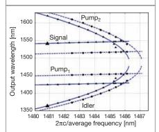
Phase-matching curves for Bragg scattering in a micro-structured fiber. Output wavelengths as functions of the average wavelength. Dashed and solid curves represent theoretical predictions, whereas circles and triangles represent experimental results with different  $P_1$ -S wavelength differences.
