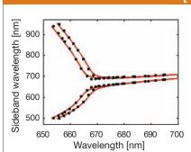
Sideband wavelengths as functions of the pump wavelength. The curves denote theoretical predictions, and the circles and squares experimental results. From A. Chen et al. Opt. Lett. **30**, 762-4 (2005).
