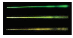
Free-space idlers generated by a 1,542-nm signal. As the pump wavelength varied from 790 to 842 nm, the idler wavelength varied from 530 (green) to 580 nm (yellow).
