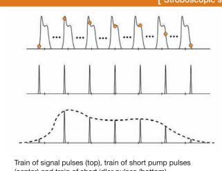
(center) and train of short idler pulses (bottom). From M. Westlund et al. J. Lightwave Technol. 23, 2012-22 (2005) and by courtesy of PicoSolve.
