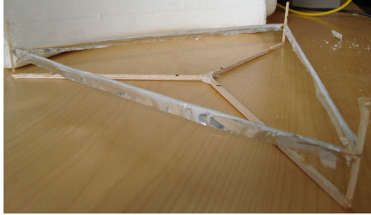
Figure 3: This is how the actual lifter looks like. Notice the “foot” which is used when measuring the lift. The corona wire can barely be seen on the figure,
