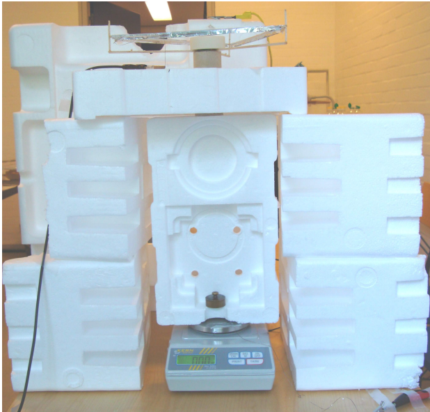
(a) Our setup of the lifter in the air test. It's seen how we have separated the scale from the lifter with polystyrene. This was to avoid high electric fields in the vicinity of the scale.
