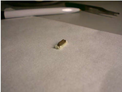
Figure 3.8: ZIF socket with kind of lock that's easy to fit the chip.
